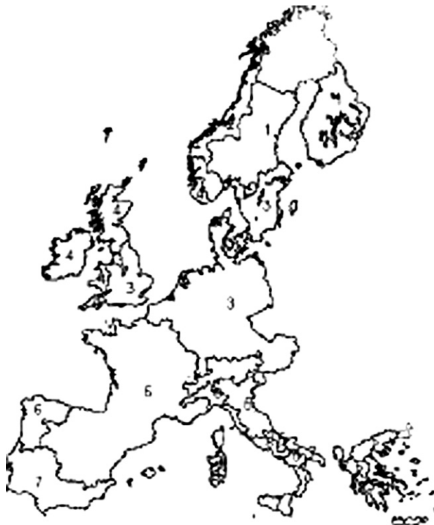
Fig. 8. The FOCUS (1997a) climatic classification for Europe. Scenarios are defined by annual precipitation excess and annual average temperature. The divisions are <400 mm, 0–5 °C (1), >400 mm, 0–5 °C (2), <400 mm, 5–10 °C (3), >400 mm, 5–10 °C (4), <400 mm, 10–15 °C (5), >400 mm, 10–15 °C (6), <400 mm, 15–20 °C (7), >400 mm, 15–20 °C.
